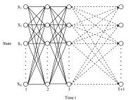
Trellis of a fully connected CRF.
