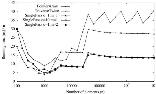
**Figure 2.** Running times of the list partitioning algorithms for  $p = 4$ .
