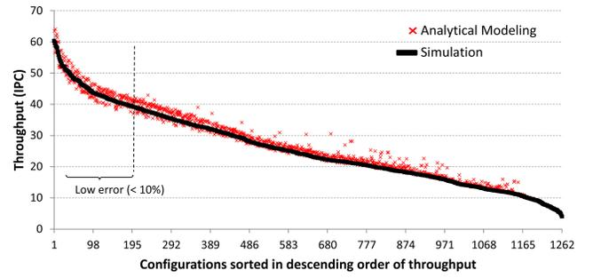
Fig. 9. Throughput comparison for analytical model and simulation.
