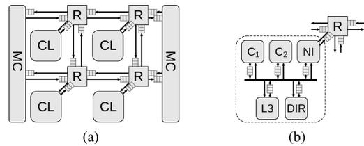
Fig. 3. Queueing model for (a) mesh NoC and (b) cluster.
