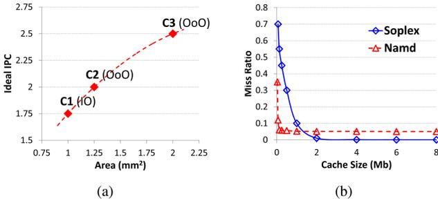
Fig. 8. Exploration setup. (a) Core types. (b) Cache miss model of *soplex* and *namd* applications.
