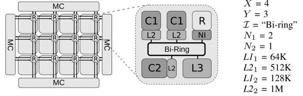
Fig. 5. Configuration example and its variables.
