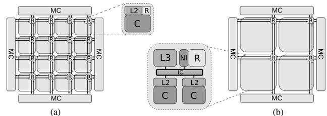
Fig. 1. CMP layouts. (a) Flat. (b) Hierarchical.
