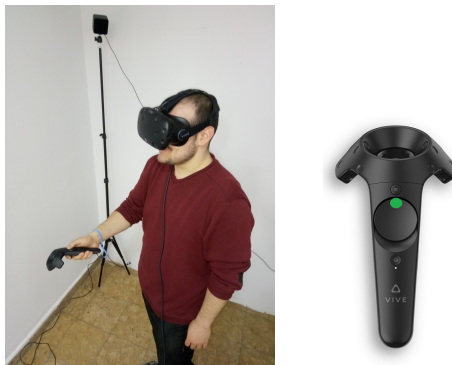
Fig. 3: On the left, participant wearing the HTC VIVE head mounted display, while interacting with the VE using the controller. On the right, controller with the green point showing where the user has to touch for walking or press for running.
