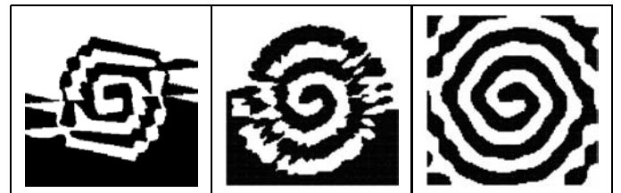
Fig. 2. Generalization obtained by Cascade-Correlation (left) and SAOCIF with logistic [-16,+16] (middle) and sine [-3,+3] (right) functions respectively for the Two spirals problem. The results for SAOCIF (with corners (-6.5, -6.5) and (6.5, 6.5) ) are the committee results.
