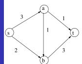
$$\begin{array}{l} \max \ f_{sa} + f_{sb} \\ f_{sa} \leq 3 \\ f_{sb} \leq 2 \\ f_{ab} \leq 1 \\ f_{at} \leq 1 \\ f_{bt} \leq 3 \\ f_{sa} - f_{ab} - f_{at} = 0 \\ f_{sb} + f_{ab} - f_{bt} = 0 \\ f_{sa}, f_{sb}, f_{ab}, f_{at}, f_{bt} \geq 0. \end{array}$$
