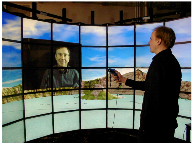
Figure 1. The Cylindrical Varrier, a high-resolution parallax-barrier autostereo VR display.
