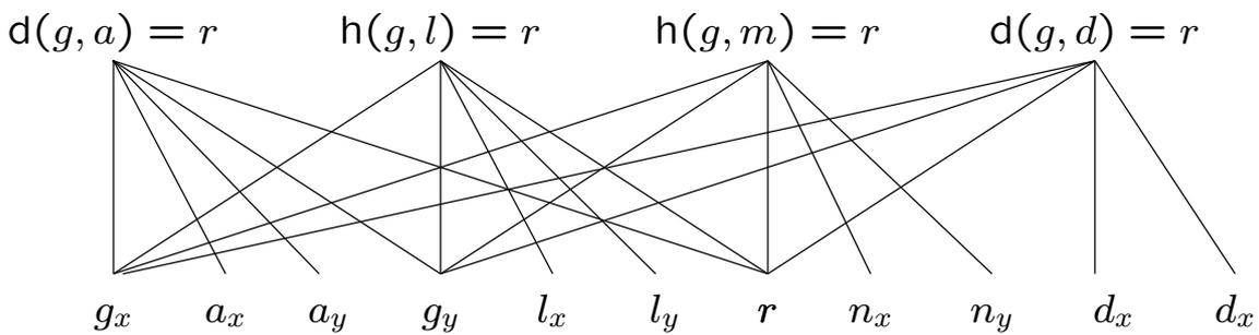
2. Compute  $R(B, C_1)$ , the *restriction* of bi-graph  $B$  by CD set  $C_1$ . The equations are analyzed with respect to a coordinate system (CD set).
