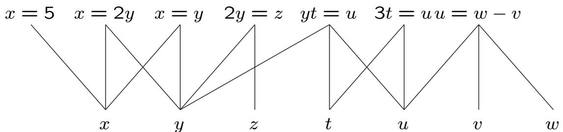
2. Compute the Dulmage-Mendelsohn decomposition of the bigraph.  $V_0$  is the over-determined part,  $V_\infty$  is the under-determined part.  $V_1, \dots, V_n$  are the consistent part.
