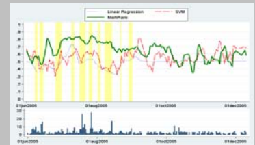
June-August 2005 performance with a weak training strategy top: performance of SVMs, MartiRank and Linear Regression algorithms measured as the normalized average rank of failures per day, new models trained every two weeks bottom: number of outages per day
