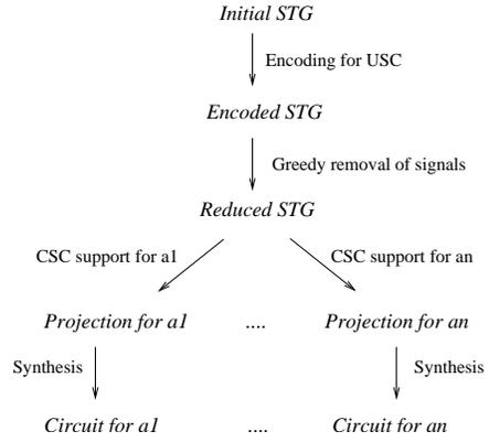
**Figure 2: Synthesis of asynchronous circuits.**
