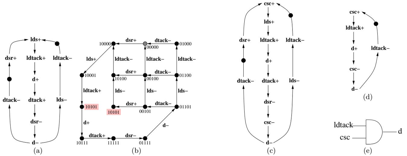
Figure 3: (a) STG, (b) State graph  $\langle dsr, dtack, ldtack, d, lds \rangle$ , (c) STG with CSC, (d) Projection for signal  $d$ , (e) Circuit implementing  $d$ .
