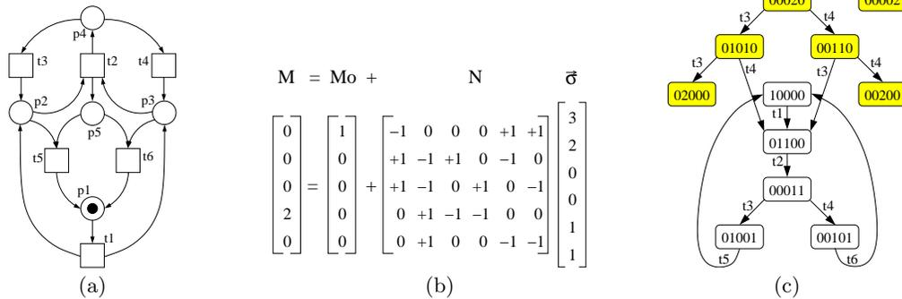
Figure 1: (a) Petri net, (b) Spurious solution  $M = (00020)^T$ , (c) Potential reachability graph.
