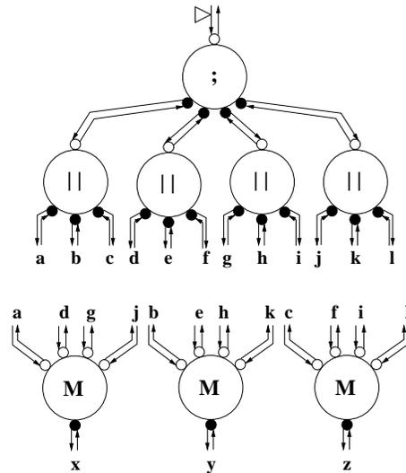
Figure 5: Netlist of handshake components from a Tangram program.
