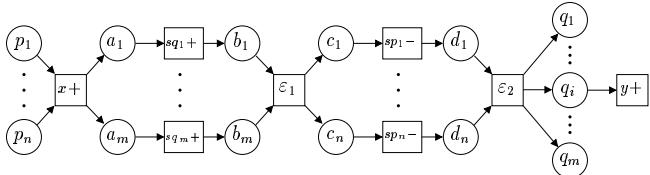
**Figure 4. Place encoding to guarantee USC.**
