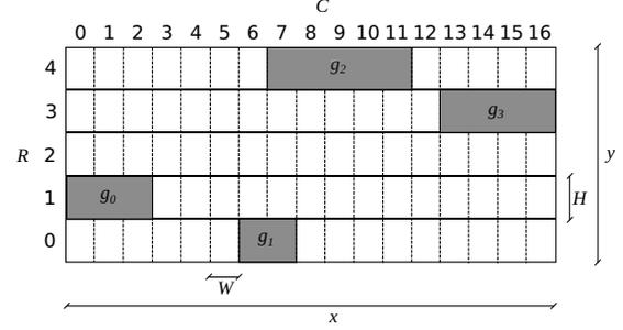
Fig. 7. Placement area for a delay line discretized into a grid.
