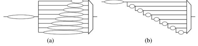
Fig. 9. Mux-based configurable RO architectures.
