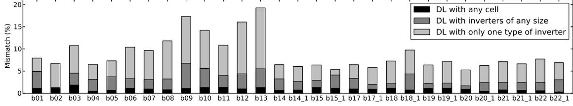
Fig. 2. Accuracy of a DL when using only inverters or any cell in the library. The Y-axis represents average mismatch.
