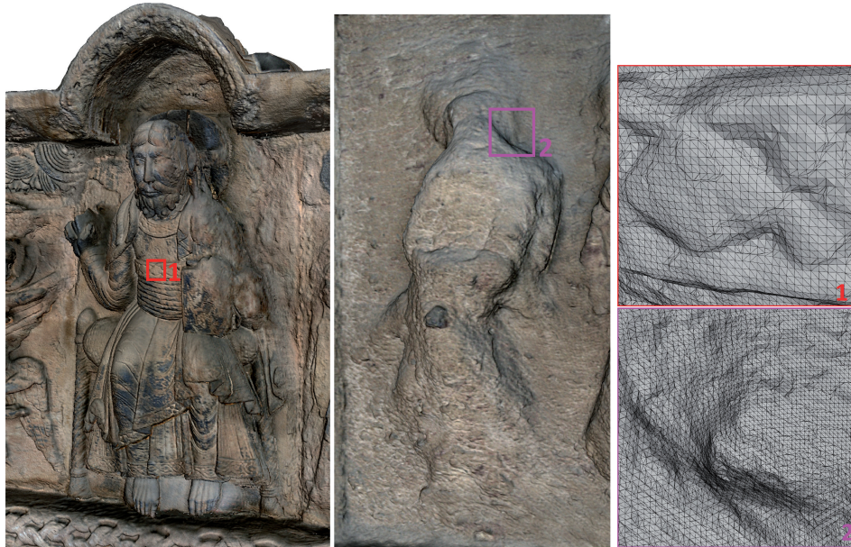
Fig. 6. Left and Middle: Two snapshots of details of the colored mesh of the Portalada. Right: Corresponding close-ups rendered with no texture and wireframe to reveal the underlying triangle mesh.
