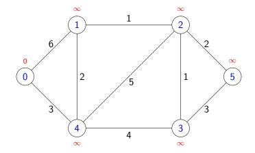
**Step 1:** associate each node with its best known distance to the source node (node 0 is the source node - the distance to itself is 0)
