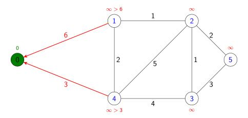
**Step 2.b:** put the selected node in the set of nodes already in the tree (green nodes); update the cost of its adjacent nodes not yet in the tree with the cost of its minimum weighted edge crossing to green nodes.
