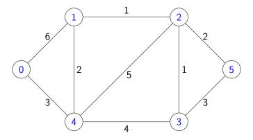
**Input:** a weighted undirected graph (with positive weights), a source node **Goal:** to compute the minimum spanning tree where source is the root node of the tree
