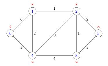
**Step 1:** associate each node with its lowest weight edge connecting the node with one already in the tree (at this stage, none of the nodes are in the tree but node 0 is the root node - fake edge with 0 cost).
