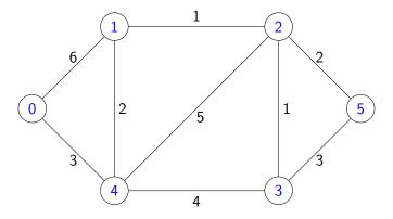
**Input:** a weighted undirected graph (with positive weights), a source node **Goal:** to compute the shortest paths from the source node to any other node in the graph
