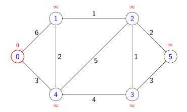
**Step 2.a:** pick the node with the lowest weighted edge crossing between green nodes (nodes already in the MST) and white nodes (nodes not yet in the MST). That minimum weighted edge is in the MST (initially, the 0-cost edge is a fake edge).
