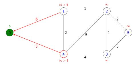
**Step 3:** repeat step 2.a (edge from node 4 to node 0 with cost 3 is in the MST) and  $\dots$
